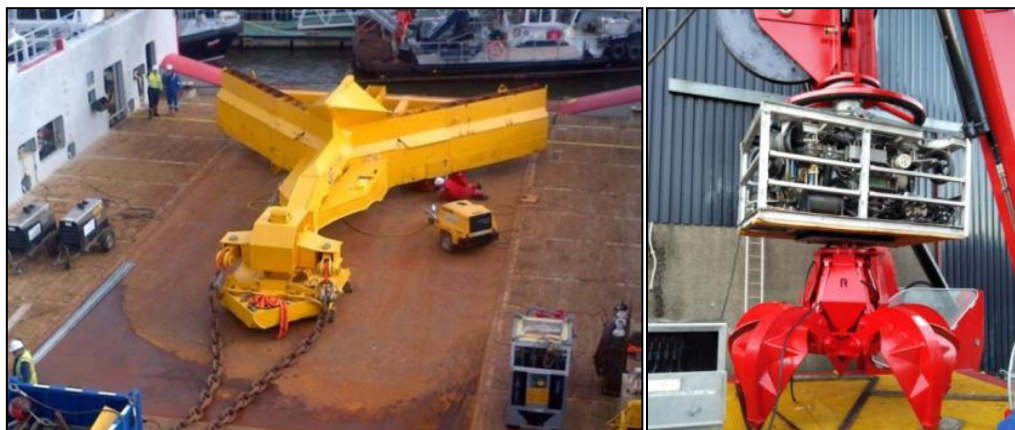
Figure 18: Plough and grapple for clearing obstacles
